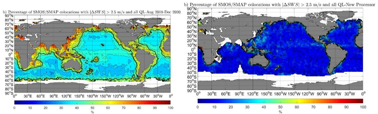
**Figure 7 : Percentage of match-up co-localized points in 2°x2° boxes between SMOS NRT and SMAP wind speeds for which the wind speed difference between the co-localized data  $|\Delta SWS|$  exceed 2.5 m/s. The thick black contour is at 50%. (left) Old processor version 110 (right) New processor version 300.**
