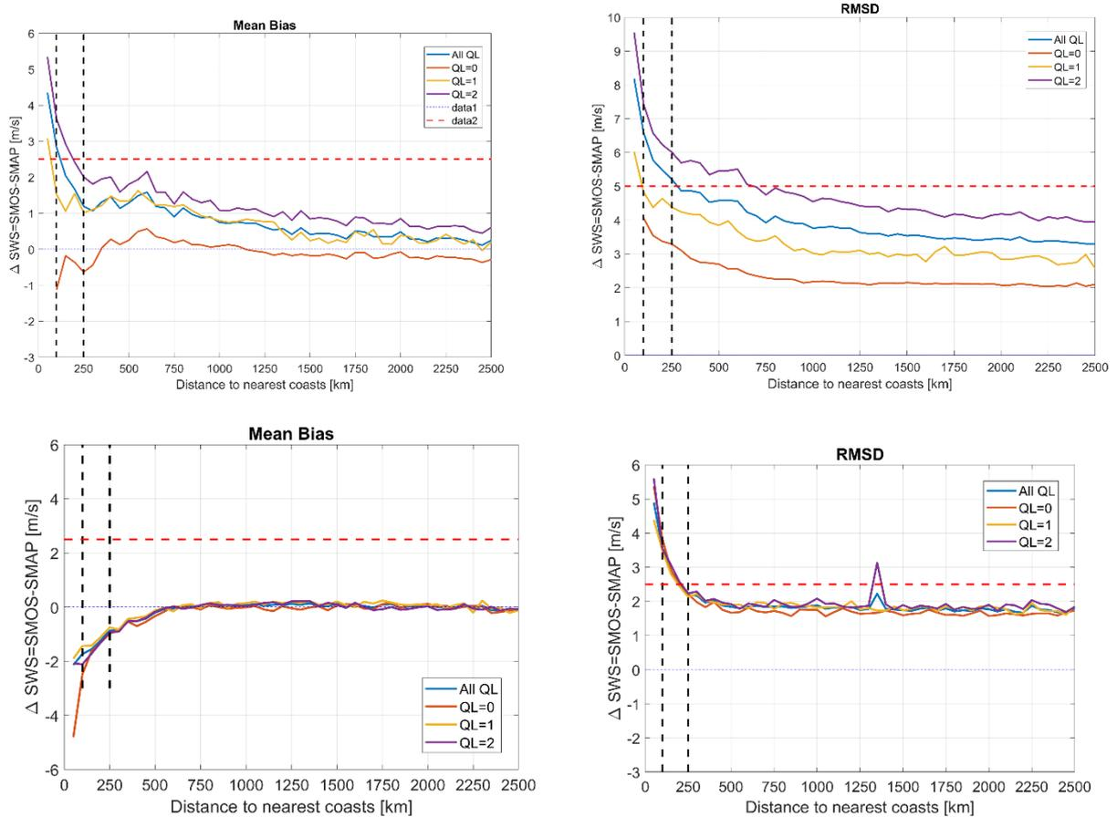
**Figure 6 : Mean (left) and RMSD (right) of the  $\Delta$ SWS (SMOS-SMAP) as a function of distance to coasts. The color indicate SMOS QL levels. Top: old processor version 110. Bottom: new processor version 300**
