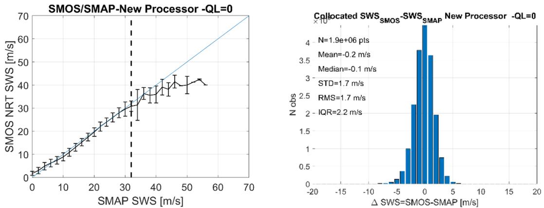
Figure 4 : (Left) Bin-averaged SMOS NRT retrieved surface wind speed as function of SMAP retrieved surface wind speed for co-located pairs (within 25 km,  $\pm 1$  hour) in August and September 2015 & 2019. The vertical bars show  $\pm 1$  standard deviation per 2 ms<sup>-1</sup> bin-width. (right) Histogram of the surface wind speed differences between SMOS and SMAP at co-localized match-up pairs. Only SMOS NRT data with Quality Level =0 (good) are accounted for.
