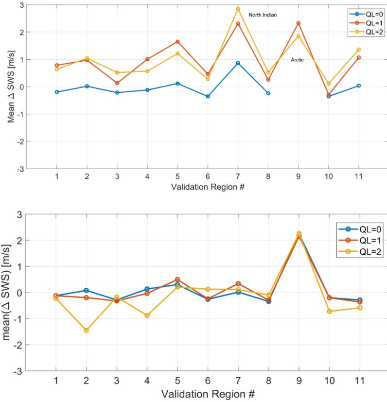
**Figure 8 : Mean bias between collocated SMOS NRT winds and SMAP winds for each validation region. The results are split as a function of the SMOS NRT wind data quality (blue is QL=0, red is QL=1 and yellow is QL=2). (top) Old processor version 110 (bottom) New processor version 300.**
