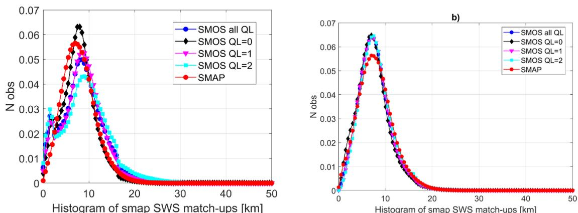
**Figure 3 : Probability Distribution Function (PDF) of the retrieved wind speed for SMOS NRT wind (blue) and SMAP (red) wind considering all the SMOS/SMAP match-ups. SWS' PDF for SMOS data with QL=0 (black curve), QL=1 (magenta) and QL=2 (cyan) are also shown. Left: Old processor v110. Right: New Processor v300.**
