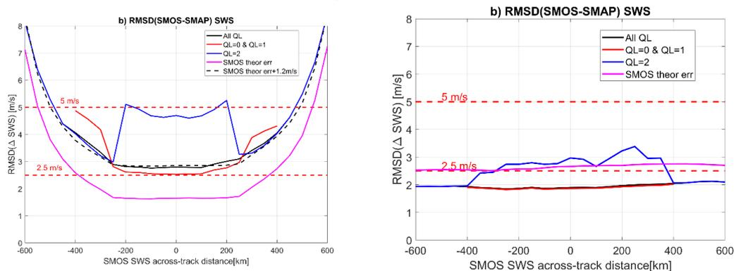
Figure 5 : RMSD of the wind speed  $\Delta$ SWS between SMOS and SMAP as a function of SMOS SWS across-track distance. The mean theoretical wind speed error provided in the NRT product is shown in magenta. The theoretical error +1.2 m/s is shown in dashed black. Left: old processor version 110. Right: new processor version 300.
